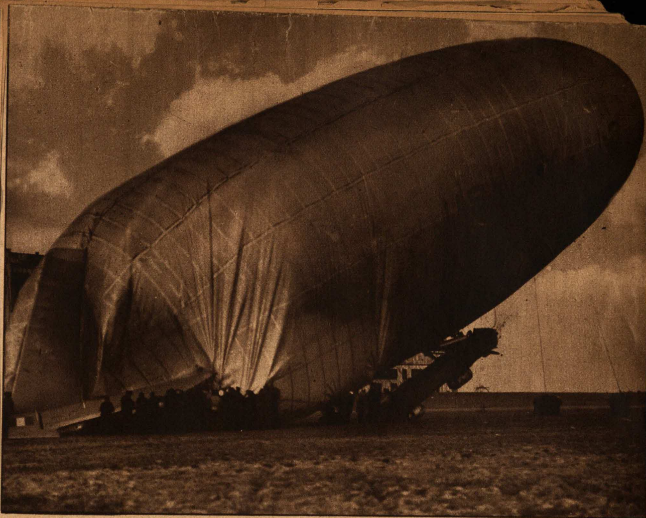
A CASUALTY WITHOUT CASUALTIES: THE NAVY BLIMP J-3, a Training Ship, Which Struck a Weather Vane in Landing and Ripped a Hole Through Which More Than 25,000 Cubic Feet of Helium Escaped, Brought to Earth Safely in Front of the Hangar at Lakehurst.
