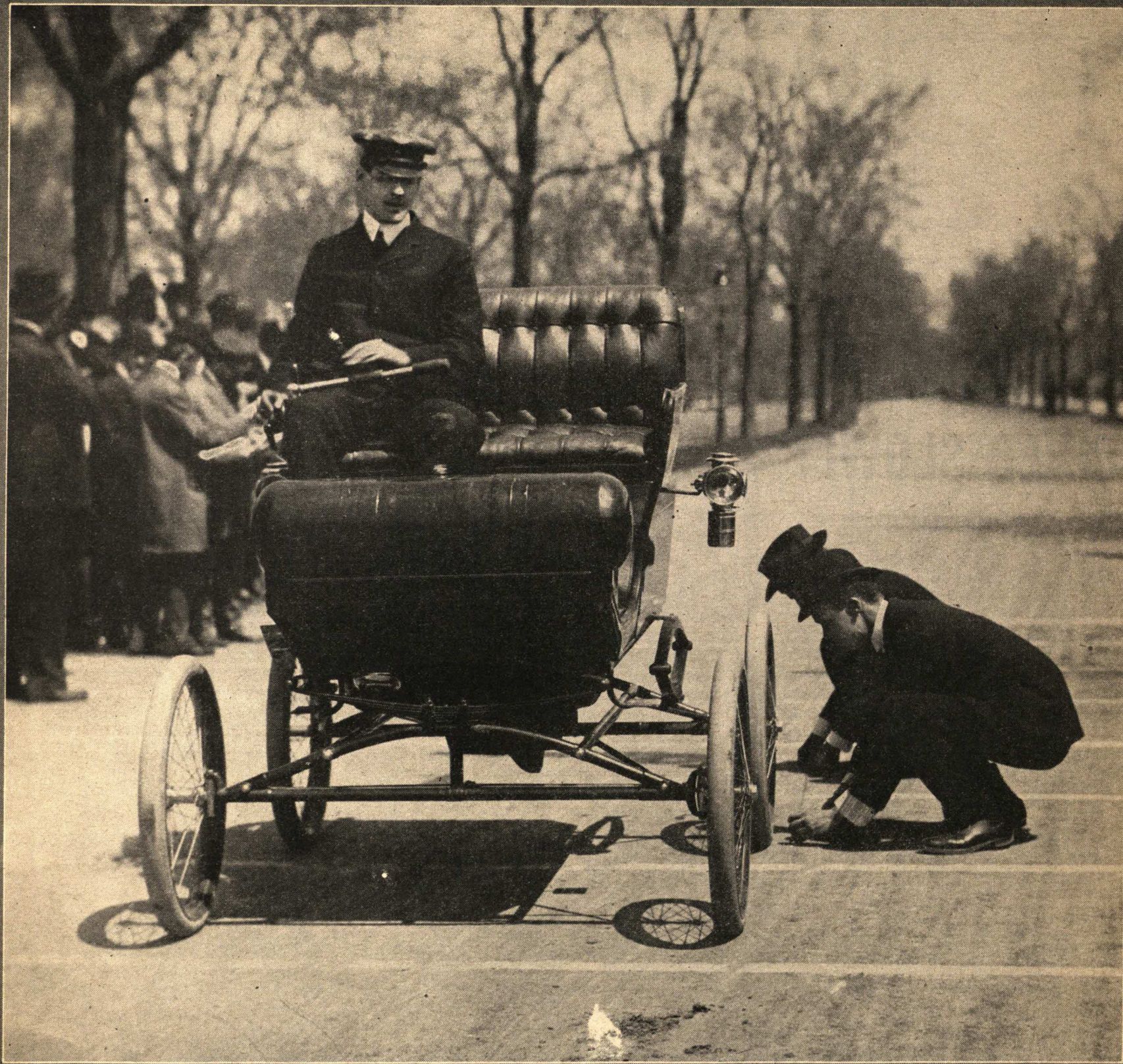
IN 1902 A LOCOMOBILE STEAMER UNDERGOES A BRAKE TEST TO PROVE THAT IT CAN BE BROUGHT TO A STOP MORE QUICKLY THAN A HORSE-DRAWN CARRIAGE
