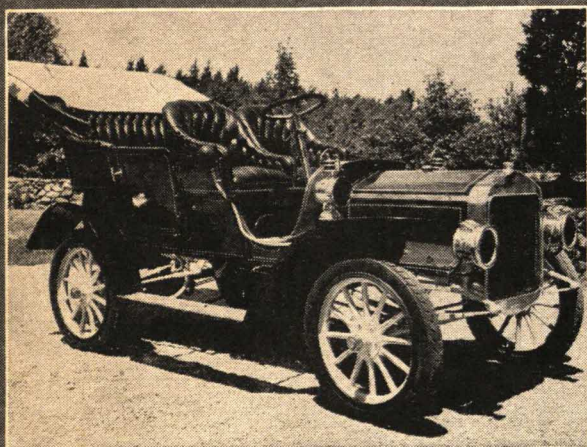
1905 BUICK touring car shows progression to the use of side door and honeycomb radiator, acetylene lights. It still employed chain drive. Cost: $1,200.
