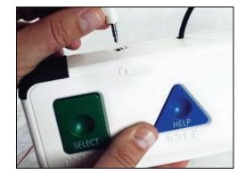
Plug the provided headphones, into the ATI's left connection port, and test them for functionality.
