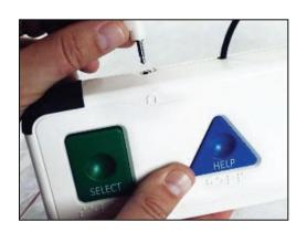
Plug the provided headphones, into the ATI's left connection port, and test them for functionality.
