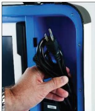
4. Use two fingers to remove the blue compartment door, retrieve the power cord and brick and replace the door.
