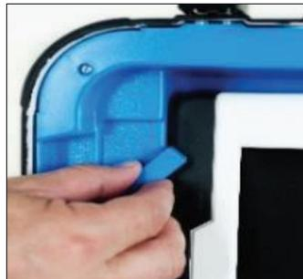
9. Use the round key color coded in black, insert it into the keyhole near the blue door and unlock it by turning the key to the left while leaving the key in place. Raise the blue latch on the upper left corner of the tablet.
