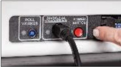
15. Press the red Power Button on the back of each Duo to power them on. It is normal for the tablet screens to go black for a short period.
