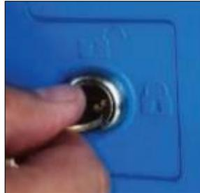
11. Tilt the tablet back, rest it against the lid, and lock it into place by turning the key to the right. A green light, on the base of the case, will illuminate indicating the tablet is correctly set. The key can now be removed.
