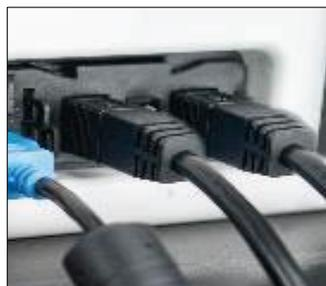
9. Grab the free end of the verity cable that is plugged into the Controller and firmly plug it into the back of the first Duo, underneath the word Verity Cables, using the left port. If the ports aren't visible, slide the cover to the right. Plug a second verity cable firmly into the second port and take that end into the left port of your next Duo. Repeat the cable steps until you have daisy chained all the Duos.
