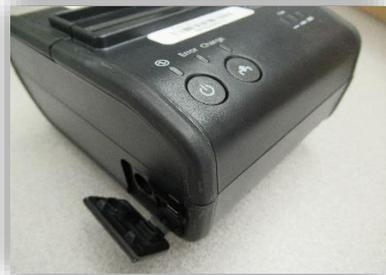
Press and hold the power button, on the lower left side, until you see the blue illuminating lights.
