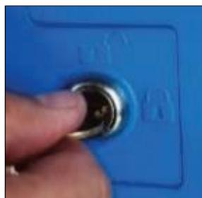
14. Tilt the tablet back, rest it against the lid, and lock it into place by turning the key to the right. A green light, on the base of the case, will illuminate indicating the tablet is correctly set. The key can now be removed.
