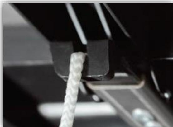
3. Reach underneath the Ballot Box lid and push the hanging cord away from you to lock the Scan into place. Confirm the Scan is secured on the box by gently lifting it from the handle.
