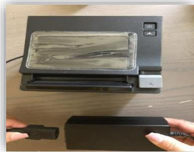
From the small portable printer, on the left bottom side, open the flap to reveal the round port and plug the power brick cord into it. Plug the remaining power cord into the brick and plug it into the power tower.
