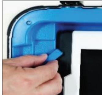
12. Use the round key color coded in black, insert it into the keyhole near the blue door and unlock it by turning the key to the left while leaving the key in place. Raise the blue latch on the upper left corner of the tablet.
