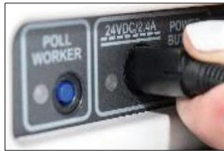
8. Plug the round end of the cord, flat side up, firmly into the back of the case in between the blue poll worker and red Power Buttons. Plug the power end into the long power strip.
