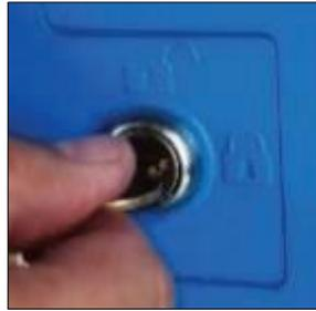
11. Tilt the tablet back, rest it against the lid, and lock it into place by turning the key to the right. A green light, on the base of the case, will illuminate indicating the tablet is correctly set. The key can now be removed.
