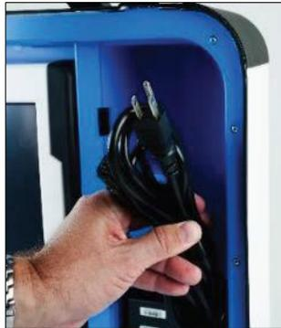
6. Use two fingers to remove the blue compartment door, retrieve the power cord and brick and replace the door.
