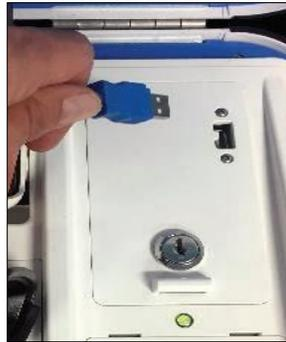
12. Retrieve the handheld barcode reader from the supply box and plug the USB end into the port on the base of the case.
