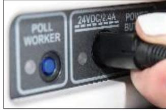
6. Plug the round end of the cord, flat side up, firmly into the back of the case in between the blue poll worker and red Power Buttons.
