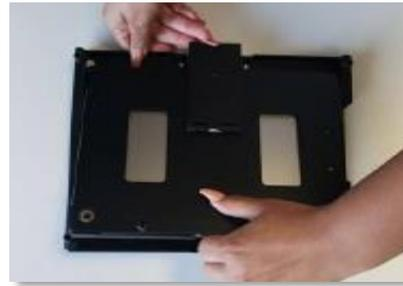
Plug smaller end of the charging cord into the port of the ePollbook, in the center of the right edge of the screen and plug the USB end into the power tower. Repeat steps for second ePollbook. Once connected to power the ePollbooks will automatically turn on.
