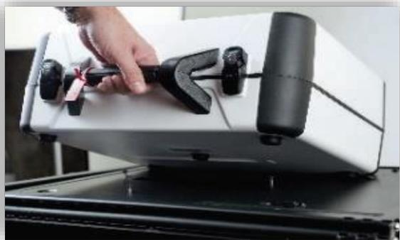
1. From the Equipment Carrier, retrieve the white case labeled with the letter "S", and place it on the Ballot Box, with the handle facing the large door of the box, while aligning the footpads on the holes.
