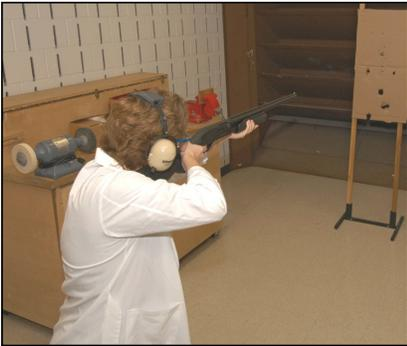
Examination and analyses of firearms, projectiles, ballistics, and markings imparted by any form of tool, fall within the purview of the firearms and tool marks laboratory. Firearms submitted are examined for inherent characteristics, unique identifiers, and safety-related factors, and can be test fired to obtain reference material that can subsequently be compared to submitted evidence. Range-of-fire determinations can be carried out on a 40-foot indoor range.
