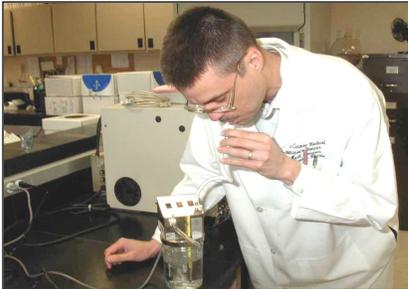
An intoxilyzer instrument provides an objective, scientific means of testing someone who is suspected by police to have been driving under the influence of alcohol by measuring a sample of the suspect's breath for determinable levels of alcohol concentration. Grant funds supplied by the Texas Department of Transportation were used to establish the ME office's intoxilyzer program in 1994. Under
